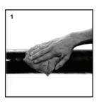
adhering paint or bad coatings are under the sealing ring. Compare the outer pipe diameter with the chucking capacity
